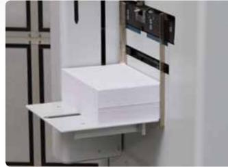
Deep pile feeder with high prestack capacity up to 4.000 sheets.
