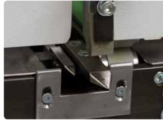
Two finger paper pick-up system allows mixed paper stocks to be handled more easily.
