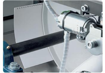
Turnover drum keeps the punched sheets in the correct page sequence and delivers them to the ejection system. Handling paperweights from 60 up to 800 gram.
