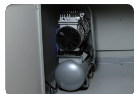
Air Compressor / Vacuum Pump
