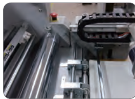
Automatic gap adjustment for feeding paper
