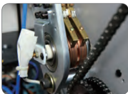
Built-in temperature sensor inside roller
