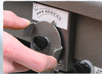
Simple dial adjustments to change from a 6 mm to a 50 mm coil.
