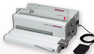
SPB 360 comfort Electric punching and electric inserting machine with manual crimping and cutting. Designed for regular use in a small to medium sized office.
